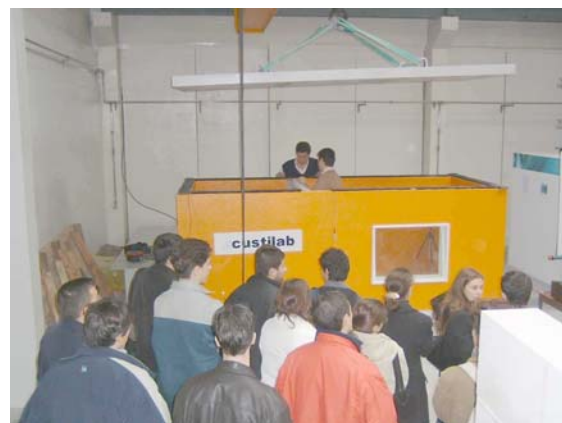
Fig. 13 - Acoustilab , a small reverberant chamber for educational purposes [2].
