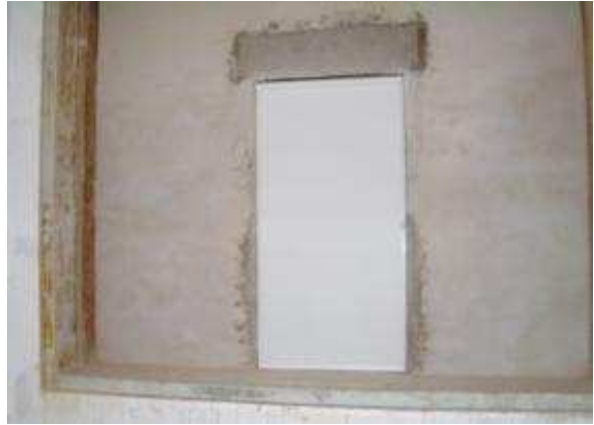
Fig. 8 and 9 – Application of the screens by the outside of the opening 8) exterior screen, half closed, on opening #1; 9) exterior screen on opening # 2, entirely closed.
