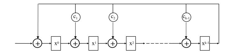
Example for the generator polynomial C(x) = x<sup>8</sup>+x<sup>2</sup>+x+1 (CRC-8 / ATM header)
