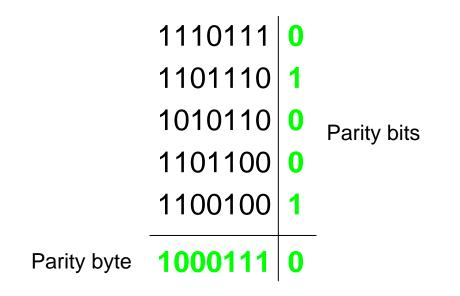
• Two-dimensional parity check detects all single bit errors, two and three bit errors and most four bit errors
