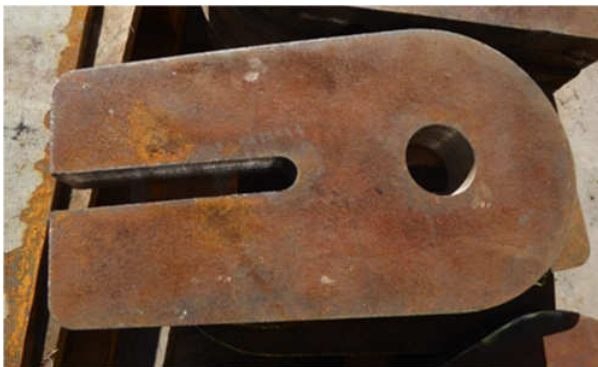
Figure 9 – New eyebars designed by Leca / Avelar
