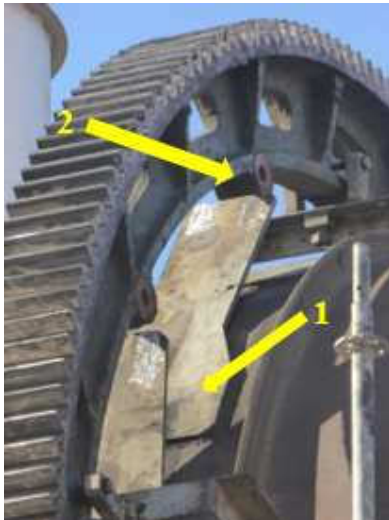
Figure 6 – Spring plates. b) Spring plate (arrow 1) connected to the kiln, but not yet connected to the toothed crown pins (the location of the pins is shown with arrow 2).
