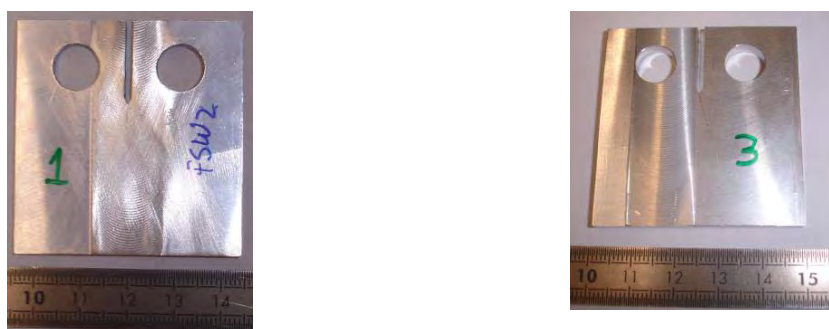
Figure – example of specimens tested, with crack in the nugget (left) and in the HAZ (right)
