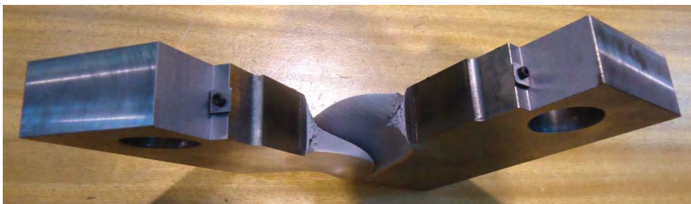
Figure – a flat surface C(T) specimen after toughness testing, exhibiting ductile rupture.
