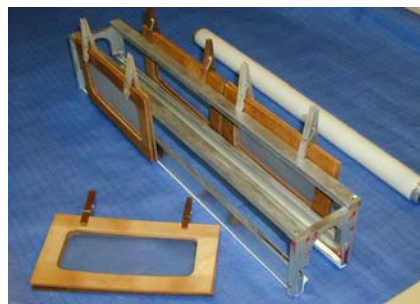
Fig. 2. Set-up for the photoageing of films.
