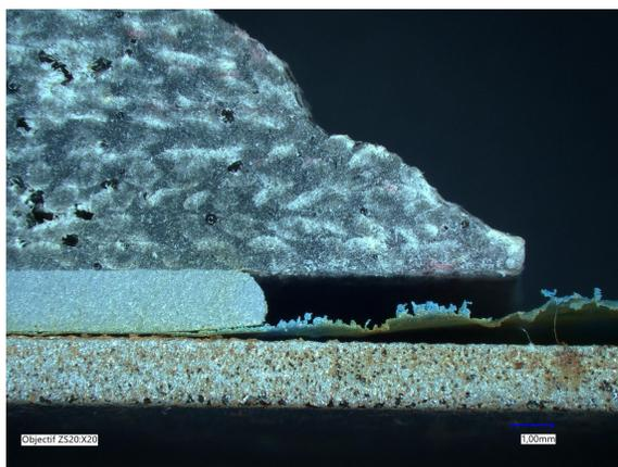
Fig. 2. Image of zone of peel initiation
