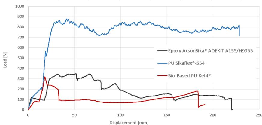
Fig. 6. Load-displacement result curves
