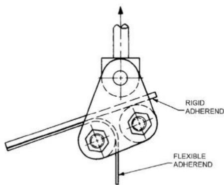
Fig. 3. Scheme of Floating roller peel test [1]
