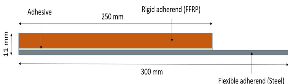
Fig. 1. Scheme of peel sample dimensions (in mm)
