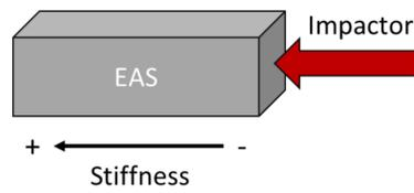
Figure 2 – Stiffness graded EAS representation.
