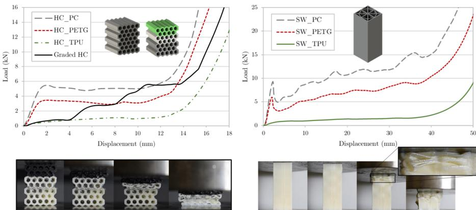
Figure 5 – Collapse behaviour of multi-material (left) and single material developed EAS
