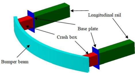
Figure 1 – Vehicle frontal energy absorption system (crash boxes in red).
