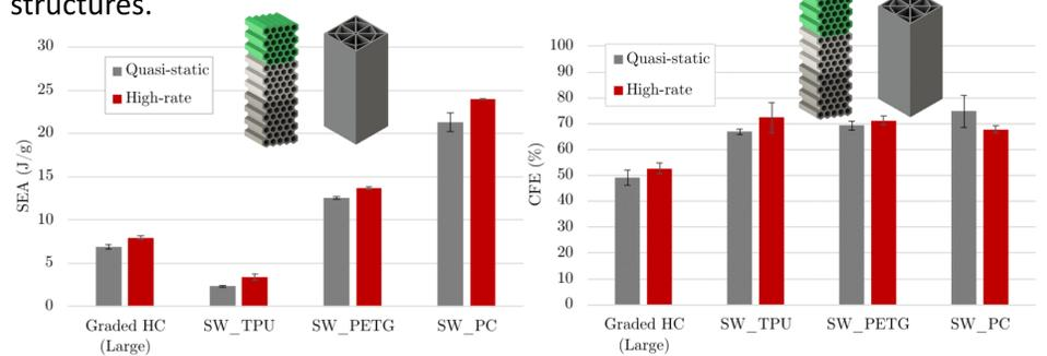
Figure 7 – Calculated SEA and CFE values for multi-material honeycomb and spider web graded structure, under quasi-static and high-rate compression.
