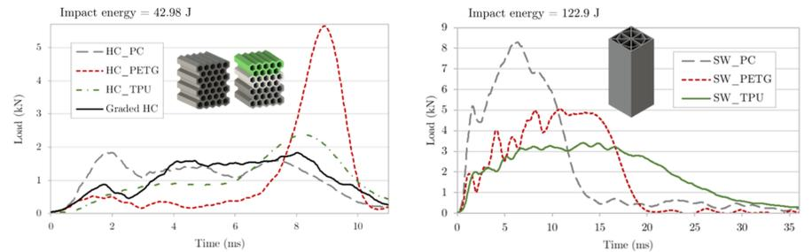
Figure 6 – Evolution of load values during the impact of the developed EAS.
