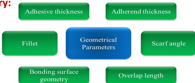
Increasing overlap length generally reduces the fatigue strength in bonded joints for the same fatigue load ratio. Strategies like fillet creation, groove patterns, and sinusoidal/zig-zag geometries on overlap surfaces enhance fatigue strength.
