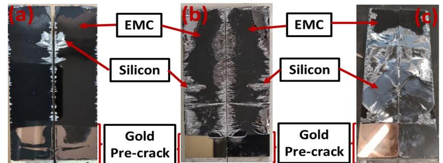
Figure 6. Typical fracture surfaces. (a) Interfacial failure. (b) Mixed failure. (c) Silicon failure.
