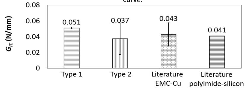
Figure 5.  $G_{IC}$  comparison with literature EMC-Cu [5-8] and polyimide-silicon [9] interfaces.
