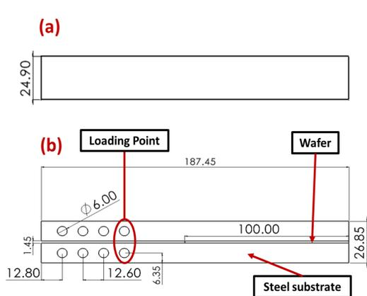
Figure 1. DCB joint geometry. (a) Top view and (b) Lateral view.
