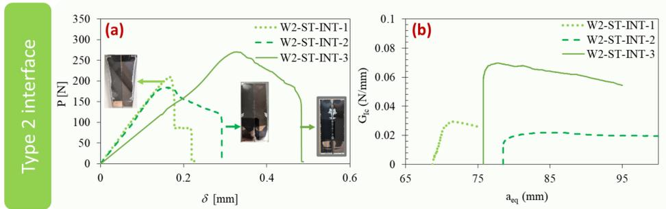
Figure 4. Type 2 interface quasi-static results. (a) Load-displacement curve. (b) R-curve.
