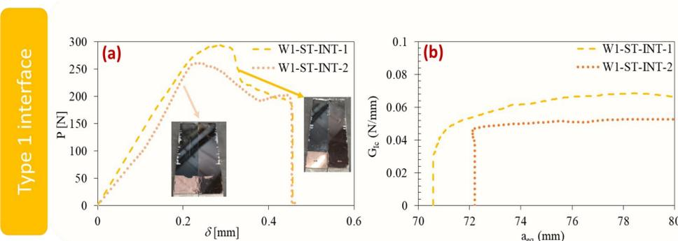
Figure 3. Type 1 interface quasi-static results. (a) Load-displacement curve. (b) R-curve.
