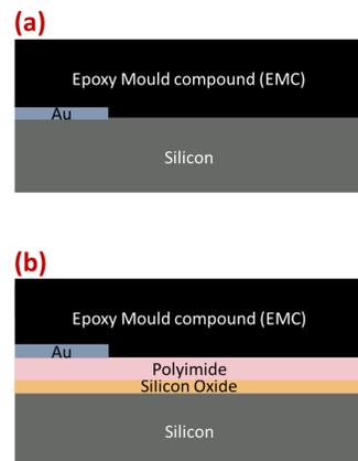
Figure 2. Scheme of (a) type 1 interface and (b) type 2 interface.
