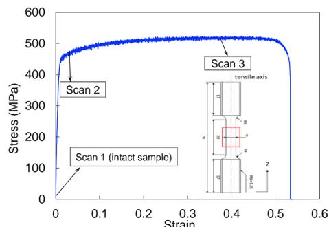
Fig. 1. Tensile stress-strain behavior of the specimen, and stress levels where XCT imaging is carried out.
