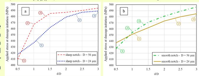
Fig. 4. Applied stress causing damage initiation in different edge distances to the pore's diameter ratio ( $d/D$ ) for two maximum and average values of the pore's equivalent diameter in the presence of (a) sharp notch (b) smooth notch with different pore sizes.
