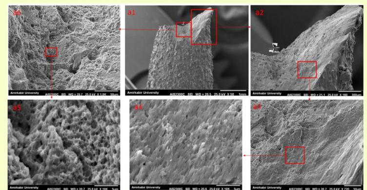
Fig. 7. Detailed SEM images from the (a<sub>1</sub>-a<sub>2</sub>) front and (b<sub>1</sub>-b<sub>2</sub>) top view of the fractured specimen.
