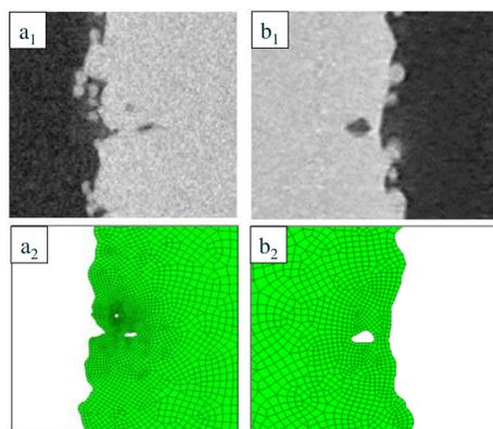
Fig. 2. Real microstructure and FE modeling of two different possible cases in the unloaded state.
