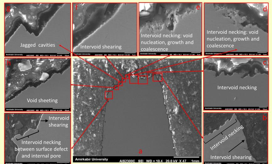
Fig. 6. Detailed SEM images of the specimen's cross-section of the fractured surface in the transverse direction showing different failure mechanisms, intervoid necking, intervoid shearing, and void shearing.
