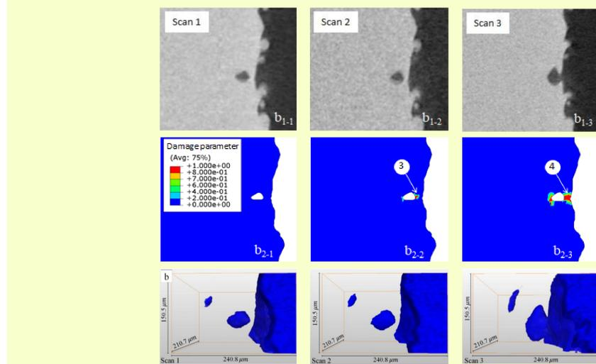
Fig. 3. XCT images and FE simulation results showing damage parameter during tensile testing for two different possible cases: (a<sub>(1-1)</sub>-(2-3)) a pore close to the sharp notch, (b<sub>(1-1)</sub>-(2-3)) a pore close to the smooth notch, and 3D XCT images.
