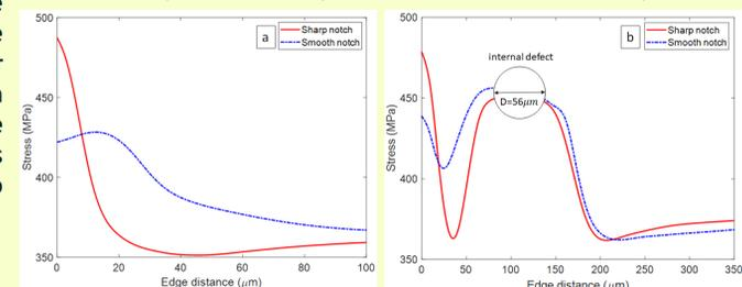
Fig. 5. The von-Mises stress distribution in the vicinity and away from the sharp and smooth notches (a) without the internal defect and (b) with the internal defect.
