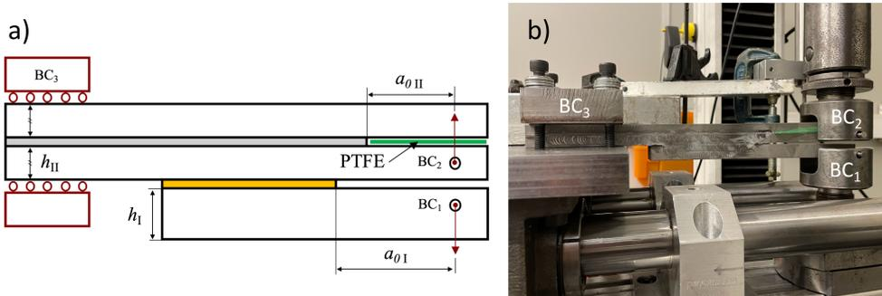
Figure 1 – Numerical and experimental apparatus. a) Relevant dimensions and numerical boundary conditions, b) experimental setup.
