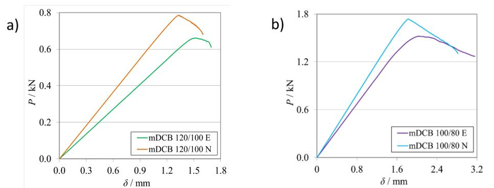
Figure 4 – P- $\delta$  curves related to the brittle (a) and tough (b) adhesives, numerical (N) versus experimental (E) results.
