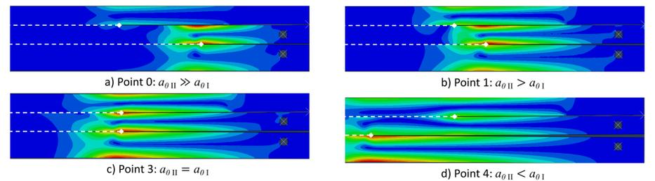
Figure 3 – Stress distributions associated with the propagation of  $a_{\theta I}$  and its passage through  $a_{\theta II}$ . The dashed white line easily identifies each adhesive layers, ELS on top and mDCB on the bottom, as well as the evolution of the crack tips.
