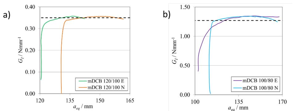
Figure 5 – R-curves related to the brittle (a) and tough (b) adhesives, numerical (N) versus experimental (E) results.
