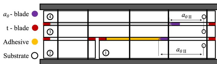
Figure 2 – Schematic representation of the stacking sequence used in experimental sample manufacturing.
