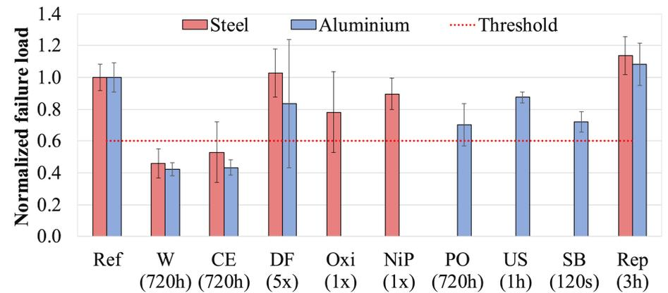
Figure 3 – Normalized shear strength of RJS joints continuously aged [2].
