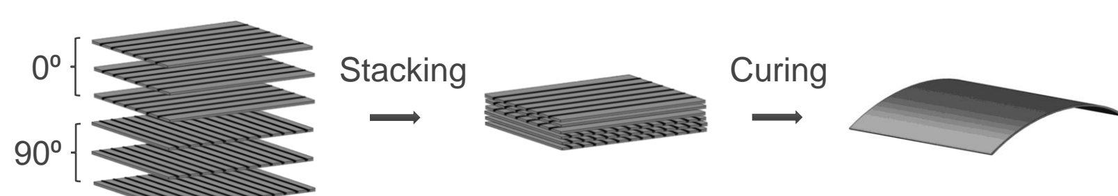
FIGURE 2. Warpage deformation in a [0^\circ/90^\circ/0^\circ/90^\circ] composite plate is caused by the orthotropic coefficients of thermal expansion.
