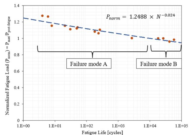
Figure 2– Normalized fatigue load vs fatigue life curve of the hole hemmed joints.
