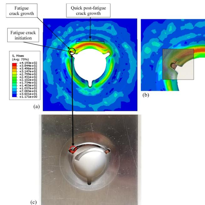
Figure 3– Comparison of the FE-predicted critical region in static analysis with the crack region observed in the experimental tests (mode B). (a) von Mises stress contour plot in the outer sheet, (b) fatigue crack from the experimental test (shown in transparency) superimposed over the von Mises stress contour plot, both scaled identically, and (c) crack propagation observed after the post-fatigue test.
