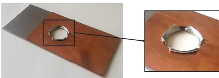
Figure 1– Novel joints between copper and aluminum busbars produced by hole hemming.
