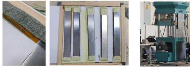
Preparation layers of laminates and ready-to-cure samples and hydraulic press
