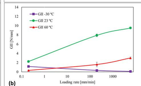
Figure 8 – Effect of temperature on fracture energy as function of loading rate for different temperatures: (a) Mode I part (b) Mode II part.
