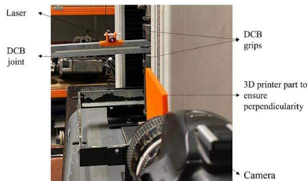
Figure 2 – DCB setup to monitor strain along the overlap and ensure perpendicularity.
