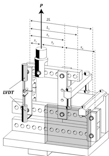
Figure 1 – Apparatus used for the mixed-mode conditions [1].
