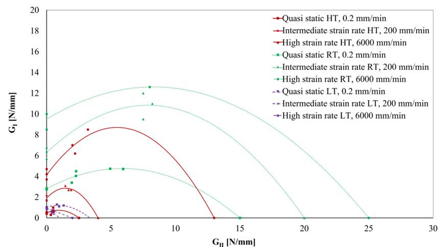
Figure 9 – Fracture envelope.
