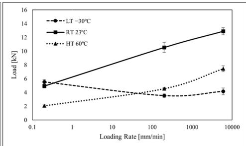
Figure 6 – Maximum load of the machine as function of loading rate and temperature for a mixed mode apparatus set up at  $45^{\circ}$ .
