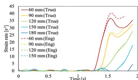
Figure 4 – True and engineering strain rates as function of time for different distances of the DCB edge (200 mm/min,  $-30\text{ }^{\circ}\text{C}$ )
