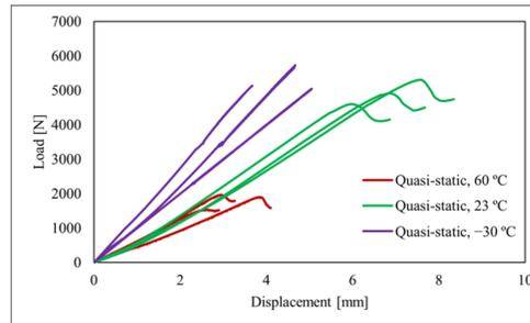
Figure 5 – Load-displacement of the machine for test submitted to quasi-static conditions for a mixed mode apparatus set up at  $45^{\circ}$ .
