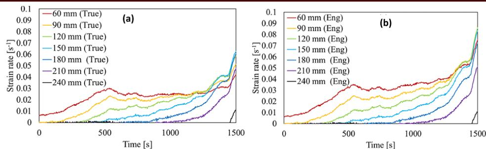
Figure 3 – True (a) and engineering (b) strain rates as function of time for different distances of the DCB edge (0.2 mm/min,  $23\text{ }^{\circ}\text{C}$ )
