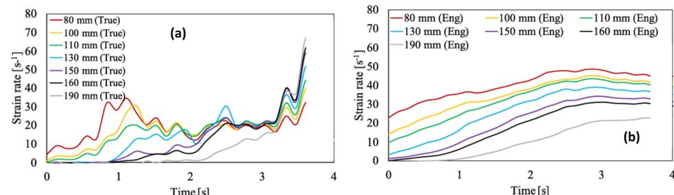
Figure 4 – True (a) and engineering (b) strain rates as function of time for different distances of the DCB edge (200 mm/min,  $23\text{ }^{\circ}\text{C}$ )
