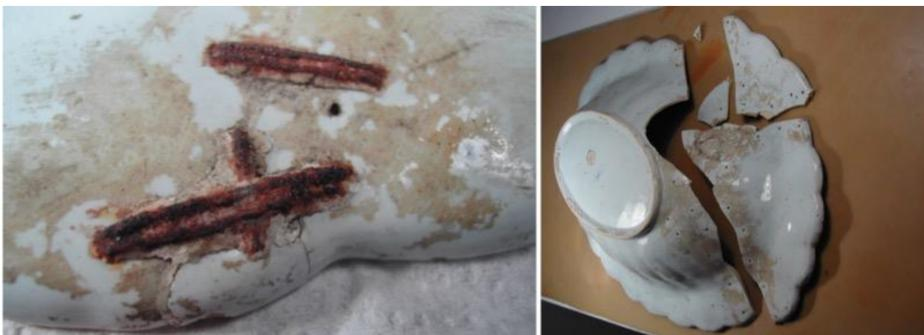
Figure 2 – Oxidized iron staples (left) and basin partially dismantled (right).
