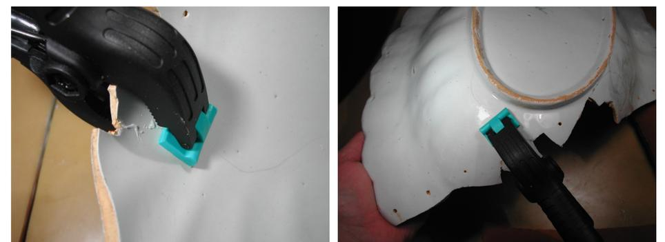
Figure 4 – Details of the bonding process resorting to clamps to ensure the correct assembly of the fragments.
