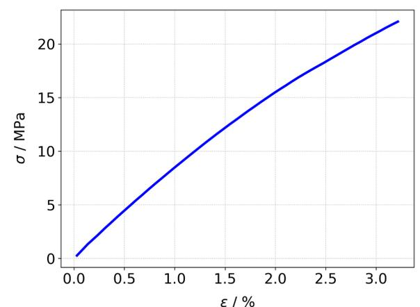
Figure 6 – Representative Stress-strain curve of the resin Paraloid B72.
