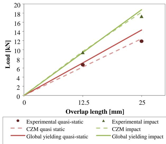
Figure 7 – Comparison between experimental, analytical and numerical results
