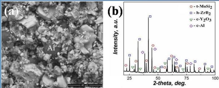
Figure 1. SEM-BSE micrograph (a) and XRD diffraction pattern (b) of the composite powder ZrB<sub>2</sub>-MoSi<sub>2</sub>-Al.
