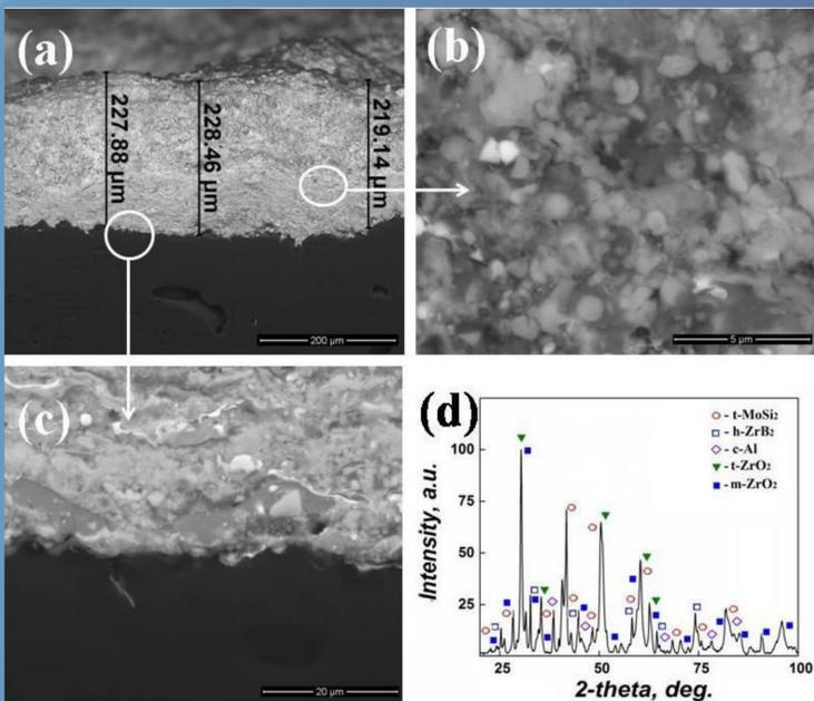
Figure 2. Cross-section SEM-BSE micrographs of the ZrB<sub>2</sub>-MoSi<sub>2</sub>-Al coating: general view (a), high magnification (b), coating-substrate interface (c), and XRD diffraction pattern.
