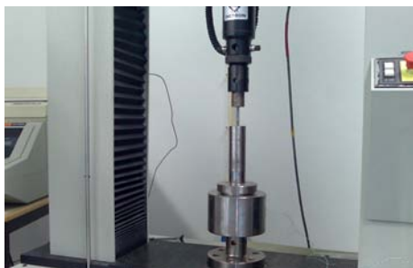
Figure 1. Instron machine with pellet's compression prototype constructed
