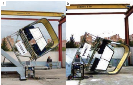
Figure 1. Roll-over test(a) and structure after the test(b).
