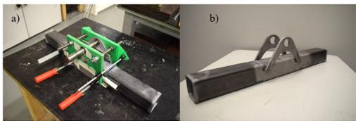
(a) Real joint during the manufacturing process. (b) A manufactured joint before the testing procedure.
