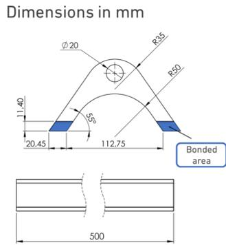
(Right): Different overlap sizes considered in adhesive bondline, (Left): Dimensions of the tab and of the tubular profile
