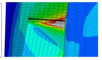
von Mises stress distribution along the weld leg, on top, total strain distribution along the weld leg, on the bottom. The applied load is 13 kN at 35° angle
