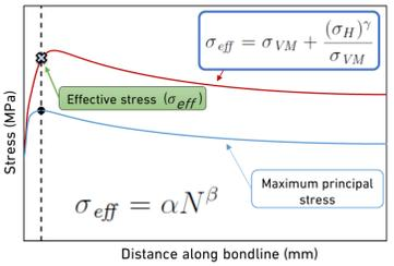
The effective stress is measured at the point where the maximum principal stress is maximum
