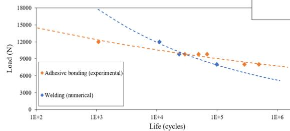
Blue. Welded joint numerical fatigue life against bonded joint experimental fatigue life.
