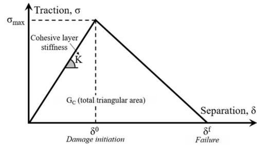
A typical triangular CZM shape used in numerical analysis of the adhesive.
