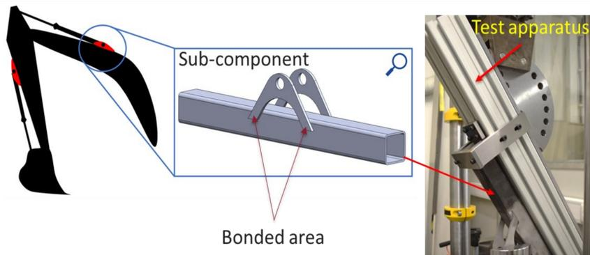
Example of a boom structure. The component analyzed in the current work is shown in the zoomed view. Apparatus mounted on testing machine at the 35° angle configuration.
