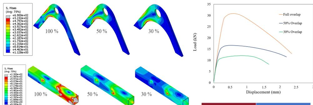
Effect of overlap length on the stress level in bonded joints
