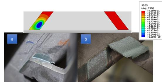
a) Plastic deformation visible as a white line on the non-failed bonded overlap. Fracture surface of the failed bonded area, under static conditions.
