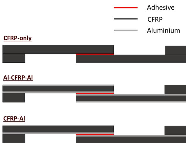
Figure 1 – Schematic representation of the configurations used.
