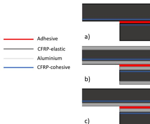
Figure 3 – Section of the numerical models used.
