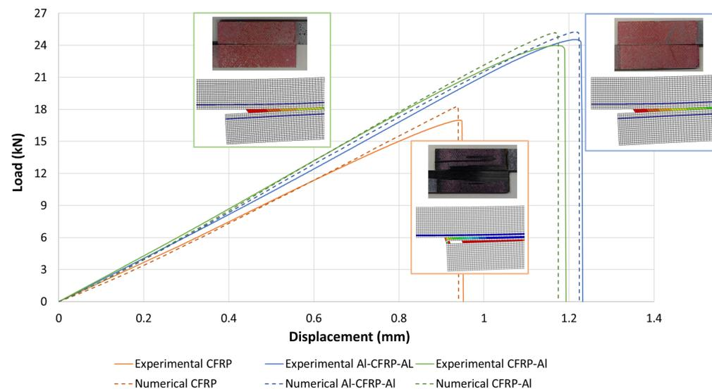
Figure 4 – Experimental versus numerical representative load-displacement curves of the different tested geometries.
