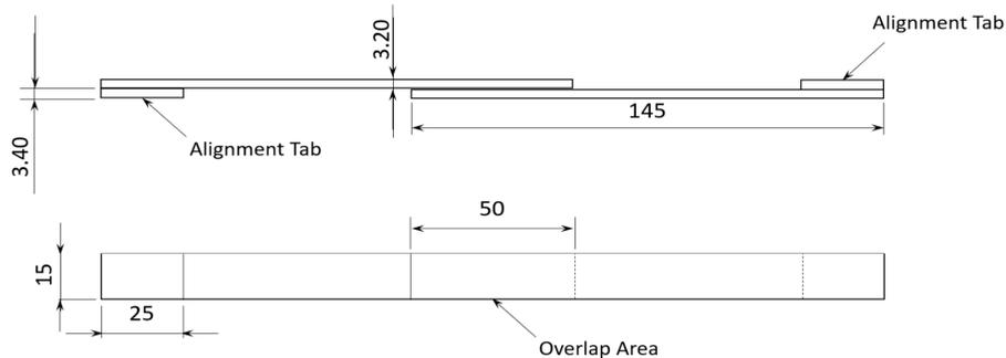
Figure 2 – SLJ specimen geometry, in mm.
